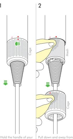
Hold the handle of your appliance firmly and rotate the filter cage anti-clockwise.
